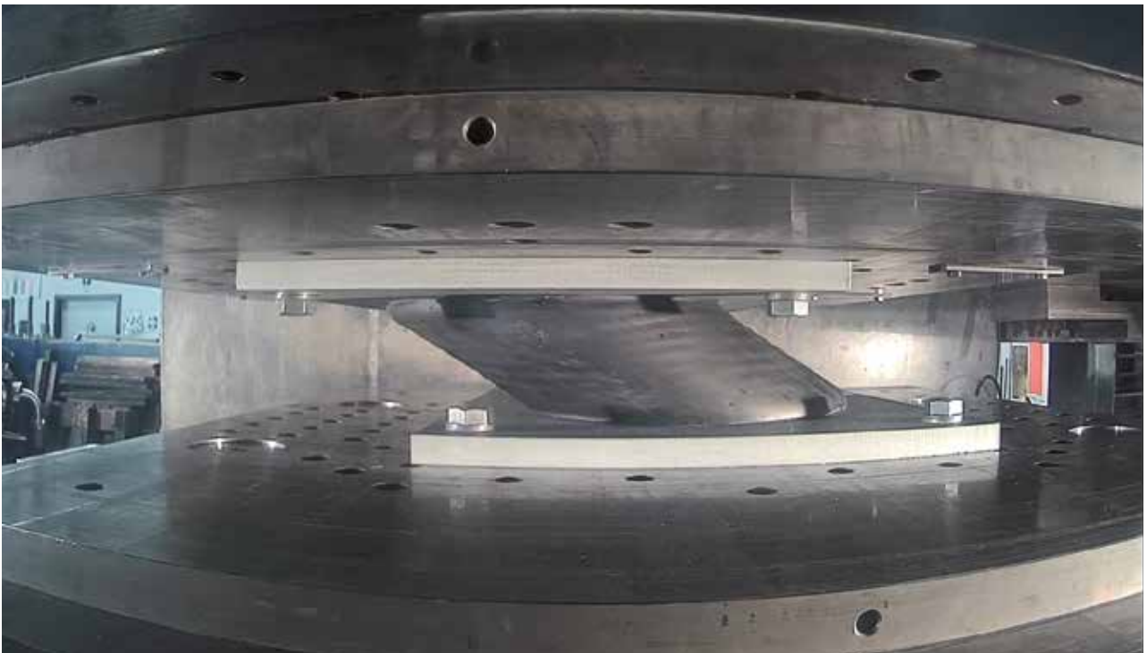
Deformed shape of LRB during testing
